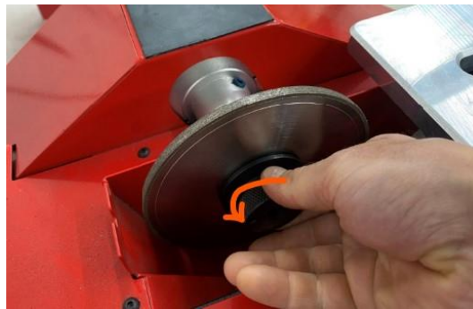
Figure 17: Tightening direction. Hold wheel with left hand and tighten knob away from table with right hand.
