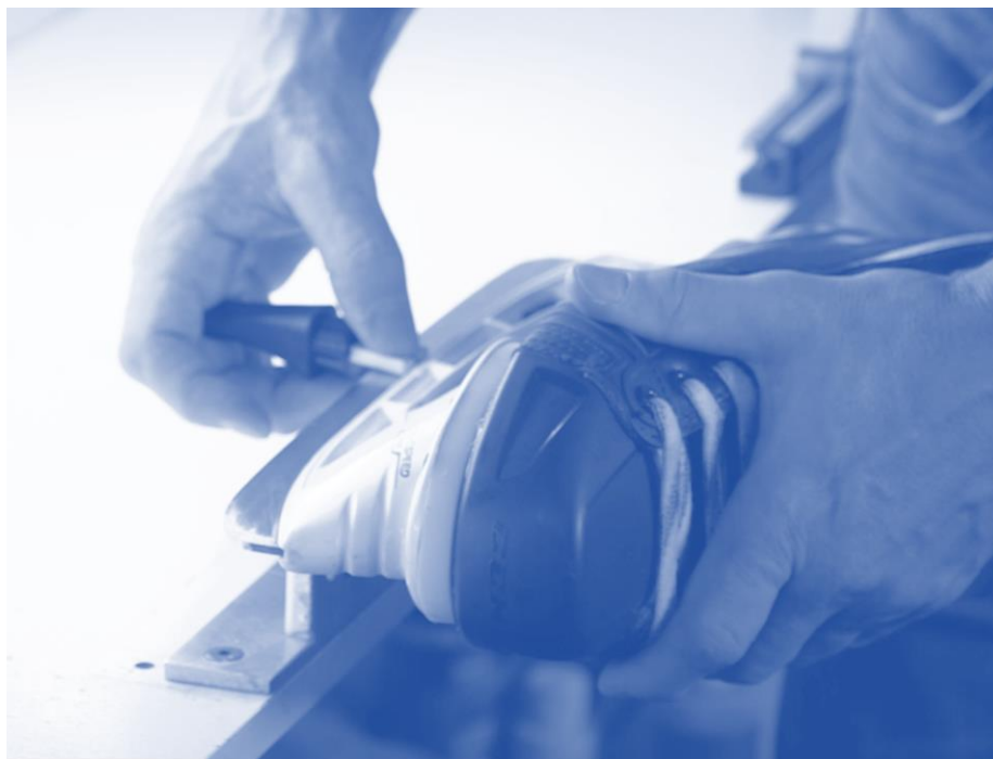
Figure 30: Stoning process. Blade well seated on blade rest. Use ceramic sweet stick on the side. Use blade side face as reference with care not to “turn the edge in”.
