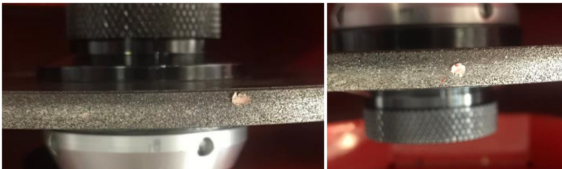
Figure 32: Small patch of metal stuck to the wheel crystal; referred to as “wheel loading”. This can be caused by poor steel quality and create vibration during sharpening. Remove by gently scratching off with metal pick or knife.
