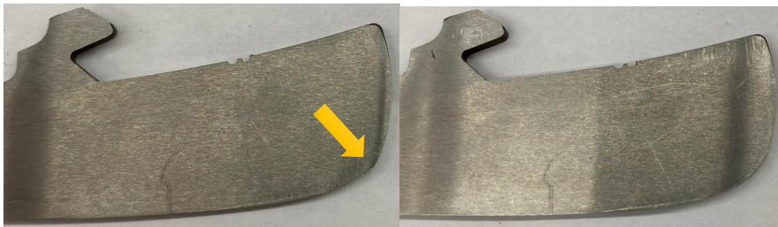
Figure 26: Typical result of using the 'Pick' option on a blade having an apex on the Heel.
