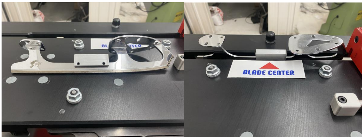
Figure 20: Mounting a figure skate blade with the provided Figure Block.
