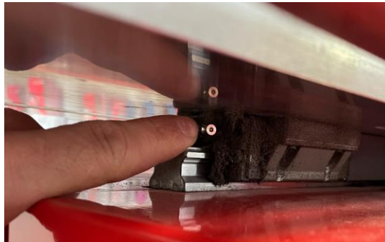
Figure 35: Grease nipple of the left-hand Linear Bearing.
