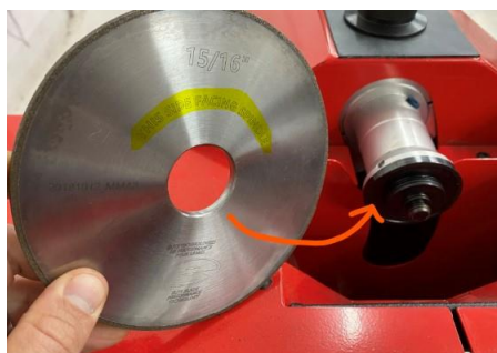
Figure 16: Proper mounting face. Wheel inscription towards spindle mounting face.
