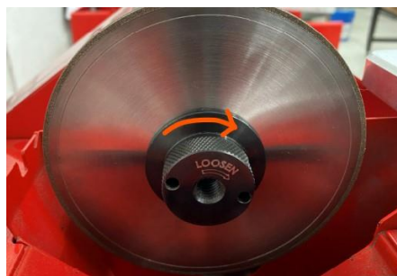
Figure 15: Loosening direction. Hold wheel with left hand and loosen knob towards table with right hand.
