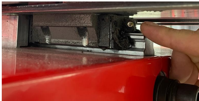
Figure 38: Right hand Linear Bearing grease nipple.
