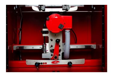
To allow even further customization of player profiles, the E-P3 has a new adjustable-pitch template mounting system, which lets the operator mount the profile template in a neutral position or in any of three progressively forward-pitched orientations (respectively 1/64", 1/32" and 3/64").
